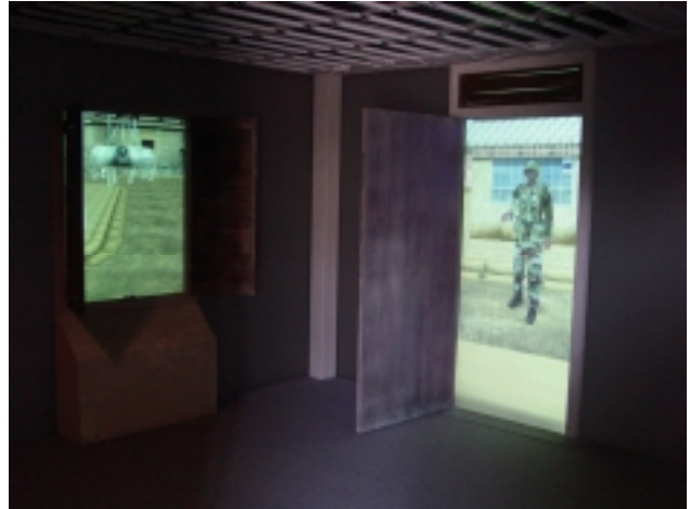
Figure 6: An OGRE based 3D graphics display client depicts views onto a city street through a physical door and window.
